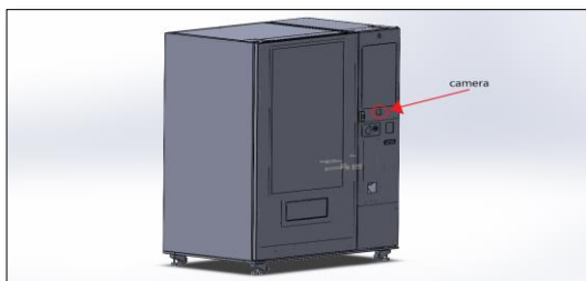
Fig. 19. 3D design of camera position on the vending machine
