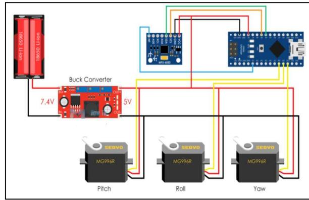
Fig. 3. Circuit connection of whole System
