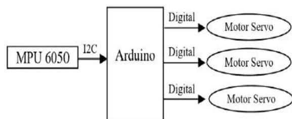
Fig. 1. Block diagram system
