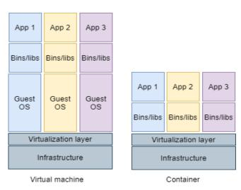
Fig. 1. Comparison of virtualization between virtual machines and containers
