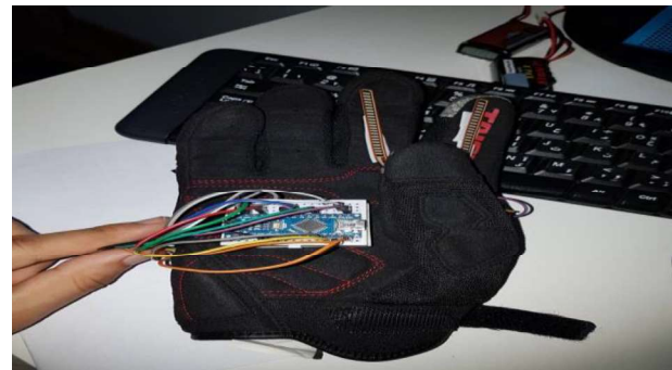
Fig. 9. Hand glove with Arduino Nano and Flex Sensors
