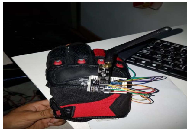
Fig. 8. Hand Glove with NRF2401 and Accelerometer
