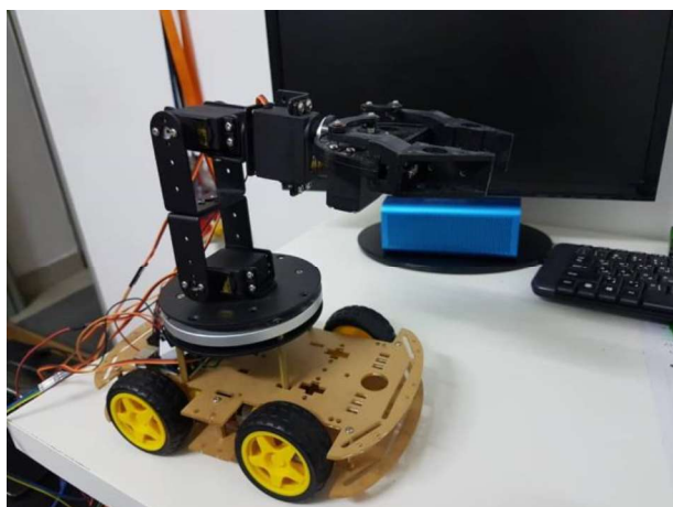
Fig. 11. The Robotic Arm with the Navigation Platform Attached
